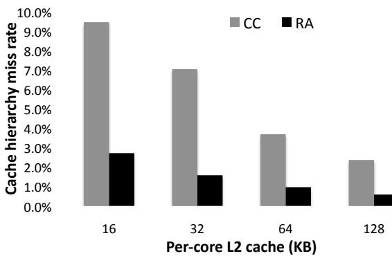
Fig. 1. Average SPLASH-2 [1] cache miss rates for various cache sizes show that duplication of shared data under CC significantly increases cache miss rates vs. RA, which does not replicate data in multiple caches. (256 x86 cores with a 16KB L1, average over the SPLASH-2 applications).
