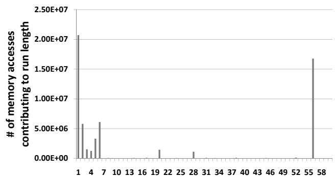
Fig. 2. The number of *non-local* memory accesses in the OCEAN benchmark binned by the number of consecutive accesses to the same remote cache (run length) highlights the weakness of RA, which pays a round-trip penalty for each remote access. (64 x86 cores with a 16KB L1 and 64KB L2 per core, hand-optimized data-to-cache assignment).
