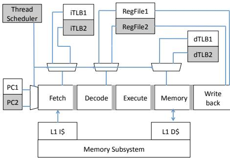
Fig. 3. An EM<sup>2</sup> core multiplexes execution among at least two contexts, each with its own architectural state. Additional state compared to a standard single-issue in-order core is highlighted in gray.
